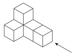
On the grid, draw the elevation in the direction of the arrow.
